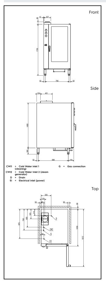
Electric Supply voltage: 260863 (EFCG22CSAS) 220-230 V/1 ph/50 Hz 1 kW **Auxiliary**: 1 kW Electrical power max.: Gas Gas Power: 50 kW Capacity: Trays type: 20 - 2/1 Gastronorm **Key Information:** External dimensions, Width: 890 mm 1215 mm External dimensions, Depth: 1700 mm External dimensions, Height: Net weight: 311.8 kg Height adjustment: 80/0 mm
